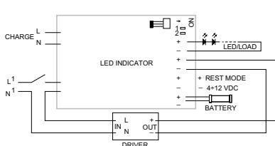
Maintained with external electronic driver diagram
