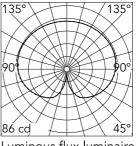
Luminous flux luminaire 1400 lm
