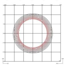
Efficiency 26.31% Coordinate System CG Total Flux 1840.50 Maximum Va**l**ue 66.01
